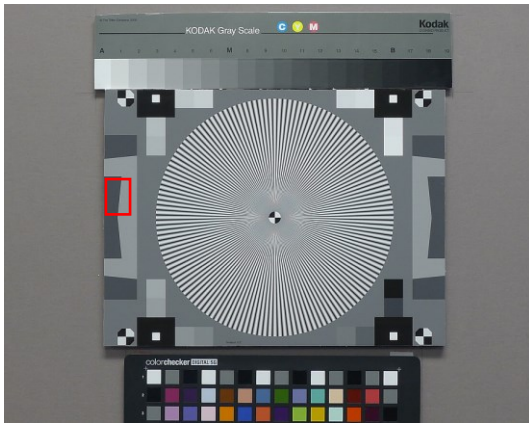
Figure 11. Typical image (cropped) including Siemens star and slanted-edges to the left and right of the star.
